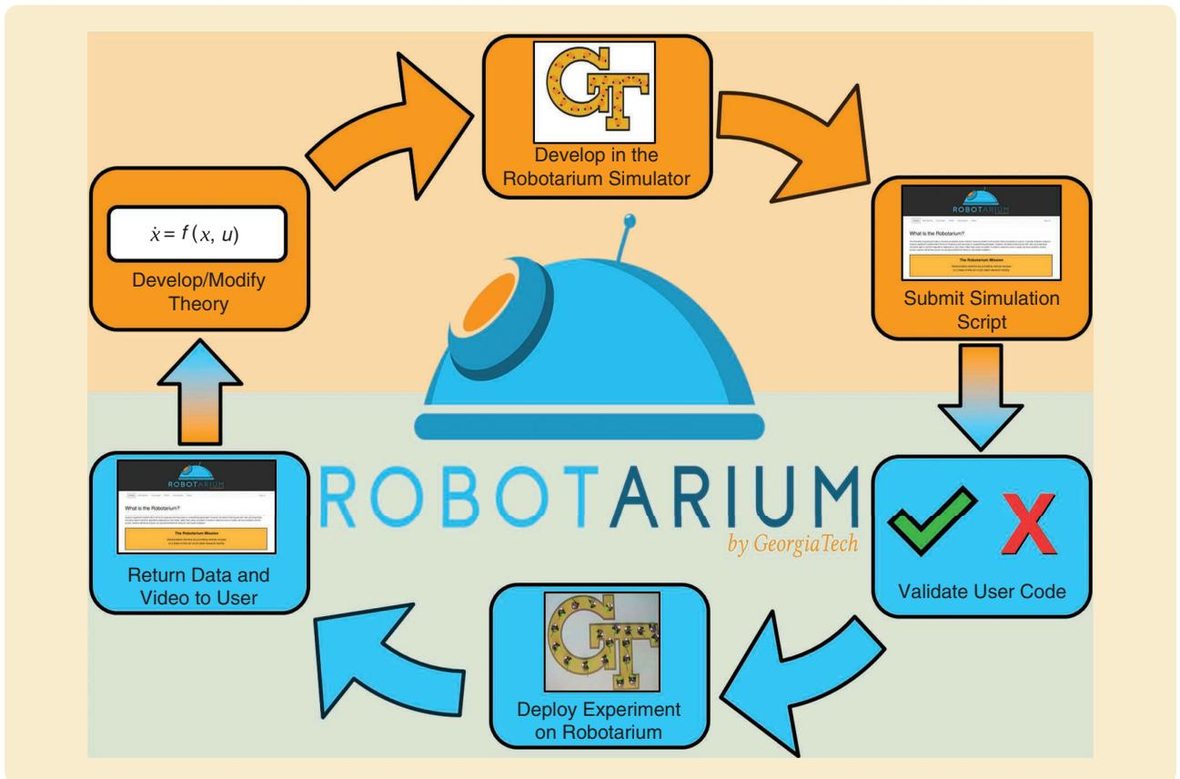
**FIGURE 5** The Robotarium submission process. The user development and submission steps are highlighted in orange, while the internal Robotarium processes are shown in blue.
