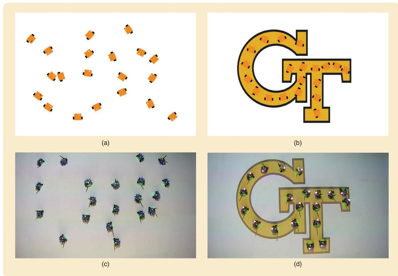
**FIGURE 4** Zoomed-in screenshots of the (a), (b) simulation and (b), (c) returned video from the Robotarium for an algorithm that drives 20 GRITSBot X robots to form the Georgia Institute of Technology logo. The (a) initial and (b) final formation of the robots in the Robotarium simulation figure. The (c) initial and (d) final formation of the robots in the deployed Robotarium experiment.
