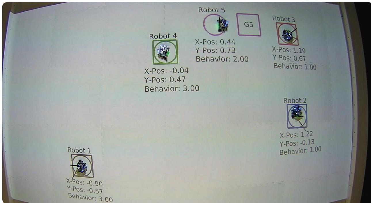
**FIGURE 3** An overhead image of an experiment on the Robotarium, which projects the simulated behavior state, number identification, and current position displayed in text around each robot. The colored squares with correlated color circles centered on each robot's current position indicate the desired goal locations for each robot.
